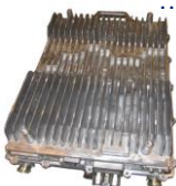
Passive cooling (cooling fins)
